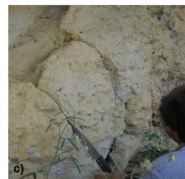
Fig. 1. a)Valle dei Templi in Agrigento: sampling area for collapsible sand, and b), c) sampling sand block by means of saw.
